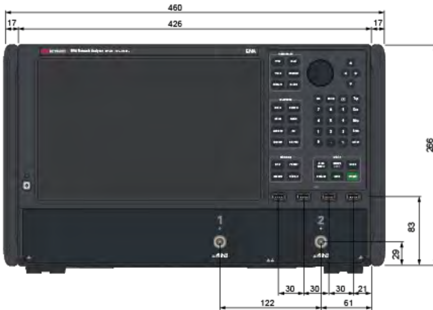
Dimensions (front view, E5080B with option 240/260/290, 2D0/2H0 + option 1NC (Type-N connectors), in millimeters)
