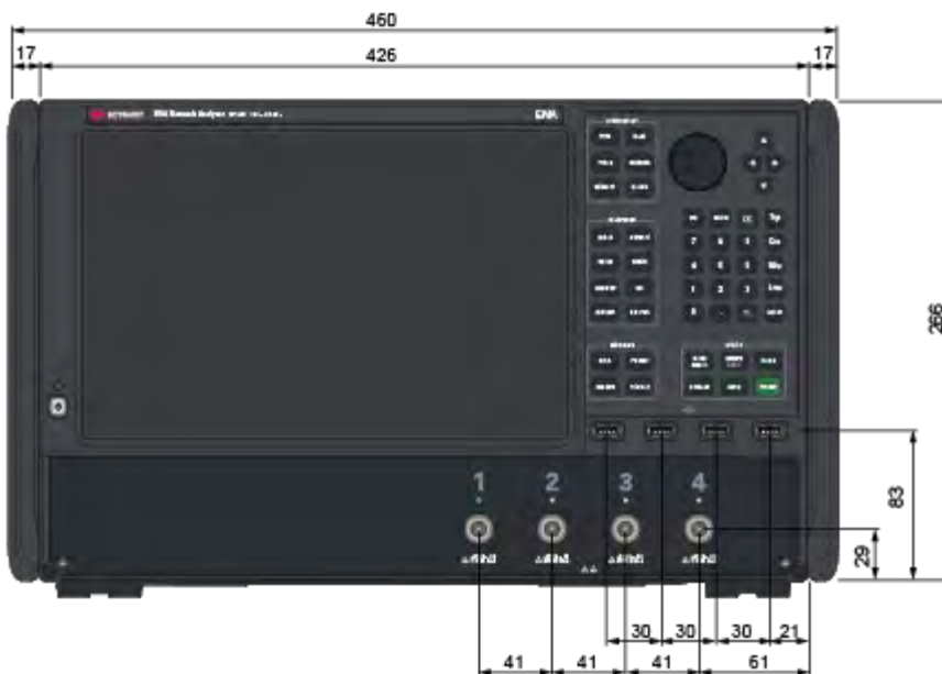
Dimensions (front view, E5080B with option 440/460/490/442/462/492, 4D0/4H0/4D2/4H2 + option 1NC (Type-N connectors), in millimeters)
